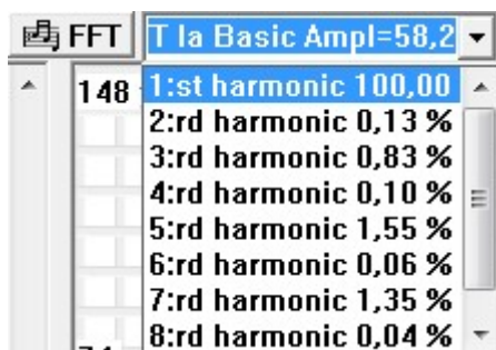
Figure 14. Harmonic Analyzer output. In this case, phase L2 has been selected and analyzed.
