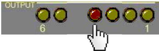
Figure 22. Moving the mouse pointer near an output LED makes it change colour which means that it is selected.
